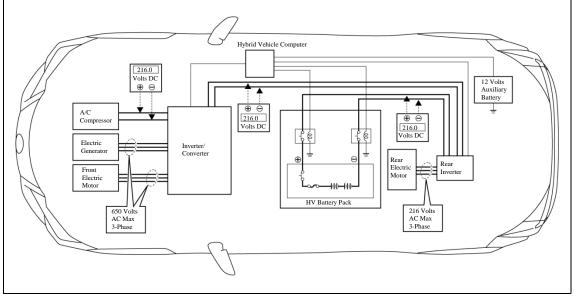
$\label{thm:eq:high-Voltage} \mbox{ High Voltage Safety System} - \mbox{Vehicle On and Operational } (\mbox{\bf READY-ON})$
