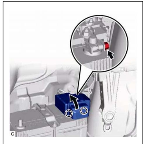
(3) Remove the nut and battery clamp sub-assembly.
