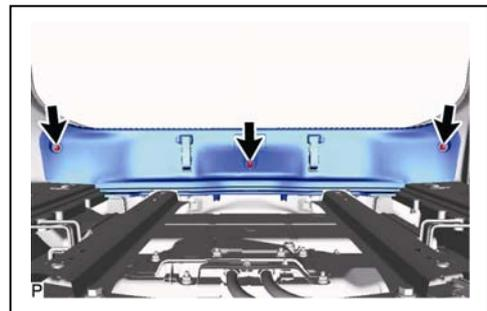
(2) Disengage the 6 clips to remove the rear luggage compartment trim cover.
