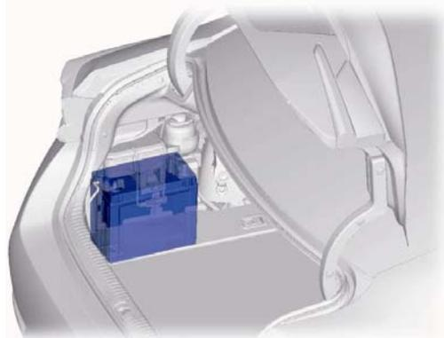
12 Volt Auxiliary Battery Mounted in Luggage Compartment Area (Left Side)
