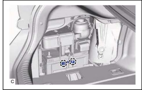
(2) Disengage the 2 guides and remove the tire repair seal from the battery clamp sub-assembly.
