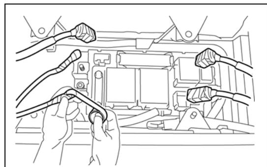
8. Check the HV battery and nearby area for leakage. If you find any liquid, it may be strong alkaline electrolyte. Wear rubber gloves and goggles and neutralize the liquid using a saturated boric acid solution or vinegar. Then wipe up the liquid using waste rags etc.
