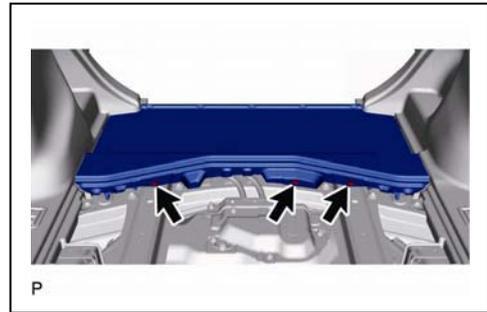
(2) Disengage the 2 fasteners and 2 guides to remove the front luggage compartment trim cover.
