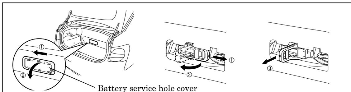
3. Carry the removed service plug in your pocket to prevent other staff from reinstalling it while you are dismantling the vehicle.
