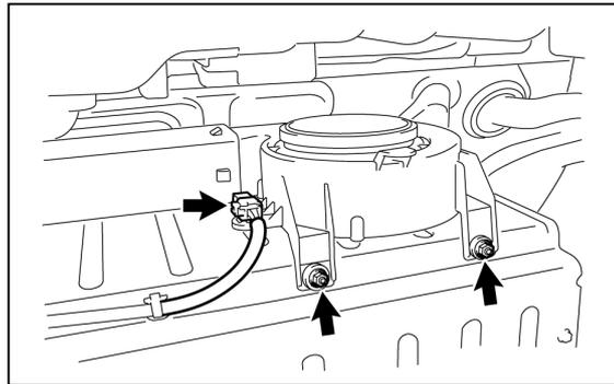
b) Separate the No. 3 HV battery intake duct from the No. 4 HV battery intake duct.
