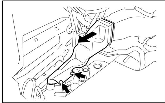
9. Remove the clips, connector clamp, and No. 1 HV battery exhaust duct.
