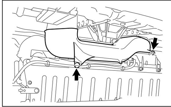
11. Remove the battery cooling blower assembly.
