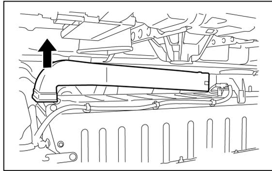
c) Remove the battery cooling blower assembly with the No. 3 HV battery intake duct from the HV battery.
