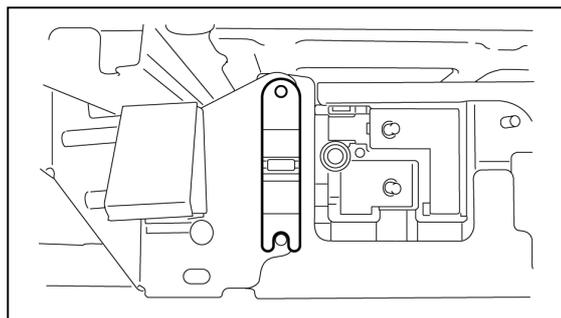
6. Remove the auxiliary battery.
