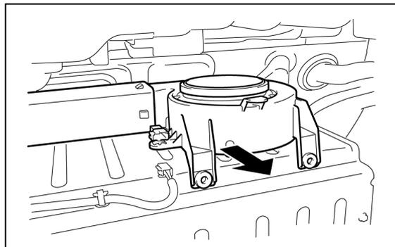
12. Remove the 6 bolts, 4 nuts, and 2 battery carrier bracket.
