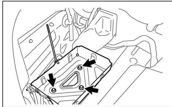
8. Remove the 2 clips and No. 2 HV battery exhaust duct.
