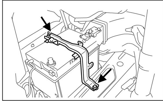
7. Remove the 3 bolts and battery carrier.
