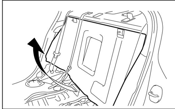
15. Remove the upper back panel corner plate RH and upper roof side inner cover.
