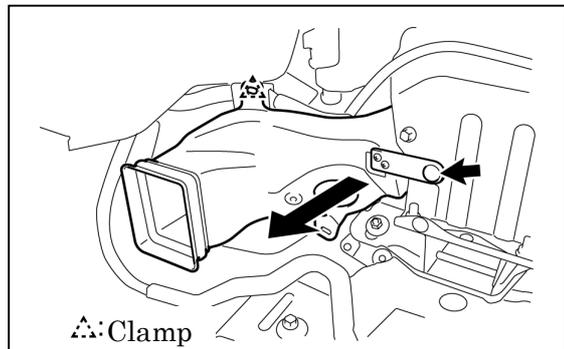
10. Remove the 2 clips and No. 2 HV battery intake duct.
