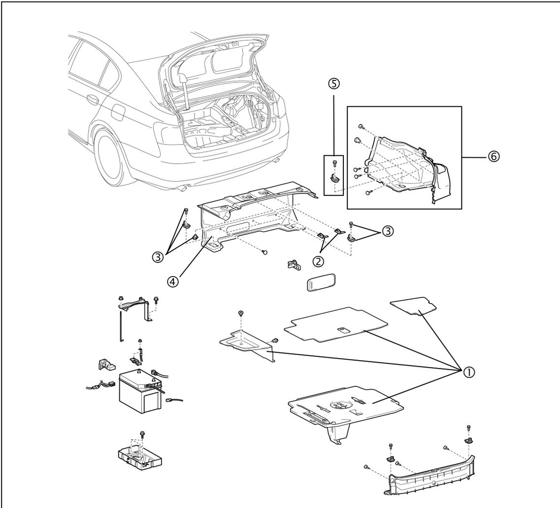
4. Remove the 2 clips and No. 3 HV battery exhaust duct.
