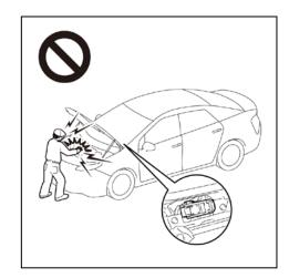
To reduce the risk of electric shock, make sure to wait at least 10 minutes after removing the service plug grip to fully discharge the high voltage capacitor inside the inverter with converter assembly.
