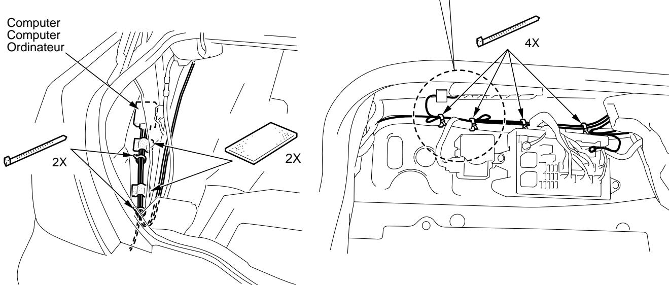
3. Gather the remaining part of the cancellation switch harness and reroute. For rerouting process, refer to Fig. 12 and 15.
