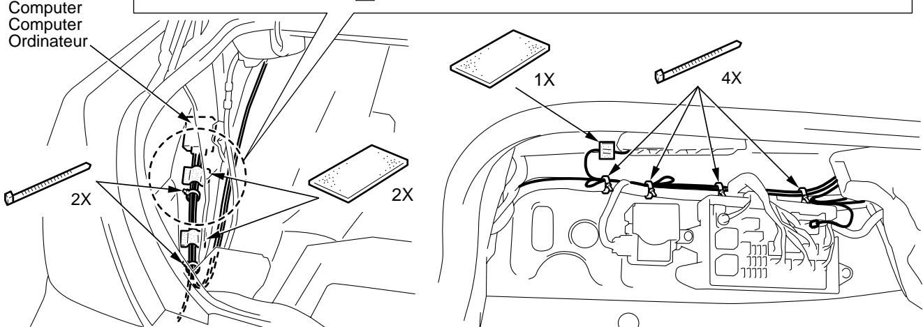
3. Refer to Fig. 10 for routing the 4 sensor harness from the vehicle interior to the outside of the vehicle interior.
